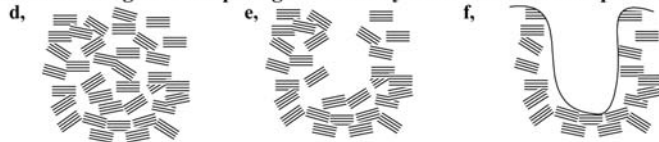
FIGURE 7 The schematic model for suggested structural change with gas activation in conventional activated carbon (a–c) and with chemical activation in novel method by KOH (d–f).
